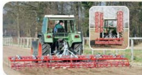
**The Platz-Max Turf** – especially developed for the use on large race courses, where a quick smoothing between several horse-racings is required. Folding by hydraulic.
