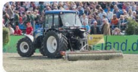
**The Platz-Max FF** – with swivelling mechanism and special roller pressing on the surface layer again. Used to maintain the variety of jumping-grounds.
