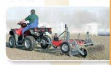
"Platz-Max Roll" – can be attached to any towing vehicle. With hydraulic adjustable chassis for easy road transport.
