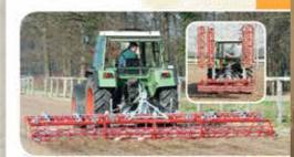
"Platz-Max Turf"— especially developed for the use on large race courses, where a quick smoothing between several horse-racings is required. Folding by hydraulic.
