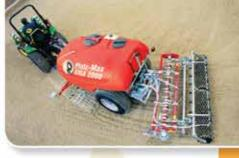
"Platz-Max Giga" – for fast levelling and watering large and little riding areas. Very manoeuvrable by special connection to the tractor. 2 hydraulic levelling units, 4 rows of water spayers to switch on/off separately (up to 180 l/min.), 3 sizes of water tanks and lot of extras.
