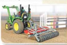
"Platz-Max FF" – with swivelling mechanism and special roller pressing on the surface layer again. Used to maintain the variety of jumping-grounds.
