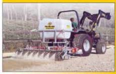
Platz-Max Rain – levelling and irrigation, all in one operation with swivelling mechanism. Flexible work outside and inside. Possibility to avoid expensive stationary watering of indoor riding arenas.
