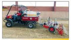
Platz-Max Roll — with optional "Rain-Module": flexible system for any towing vehicles with a little loading space for the water tank. Special appliances allow diverse other vehicles also carrying a tank, top.
