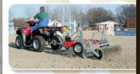
**The Platz-Max Roll** – can be attached to any towing vehicle. With hydraulic adjustable chassis for easy road transport.
