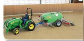
The Platz-Max Giga — for fast levelling and watering large and little riding areas. Very manoeuvrable by special connection to the tractor. 2 hydraulic levelling units, 4 rows of water spayers to switch on/off separately (up to 180 l/min.), 3 sizes of water tanks and lot of extras.
