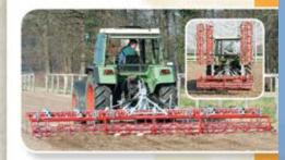
"Platz-Max Turf"— especially developed for the use on large race courses, where a quick smoothing between several horse-racings is required. Folding by hydraulic.
