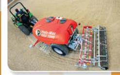
"Platz-Max Giga"— for fast levelling and watering large and little riding areas. Very manoeuvrable by special connection to the tractor. 2 hydraulic levelling units, 4 rows of water spayers to switch on/off separately (up to 180 l/min.), 3 sizes of water tanks and lot of extras.
