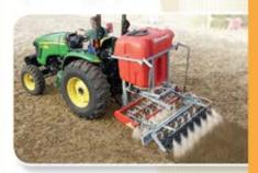
"Platz-Max Rain" – levelling and watering, all in one operation with swivelling mechanism. Working flexible inside and outside.
