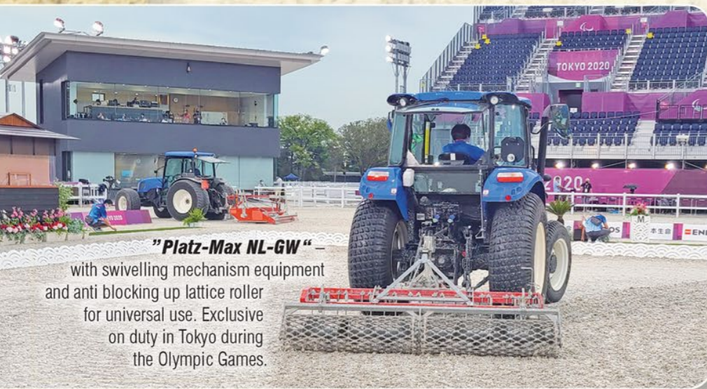
"Platz-Max Multi" – universal leveller for maintenance of nearly all riding surfaces. The smoothing board and roller operate alternately by hydraulic mechanism.
