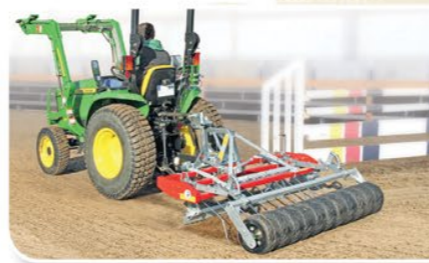
"Platz-Max FF" – with swivelling mechanism and special roller pressing on the surface layer again. Used to maintain the variety of jumping-grounds.
