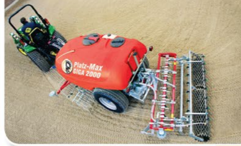
"Platz-Max Giga" – for fast levelling and watering large and little riding areas. Very manoeuvrable by special connection to the tractor. 2 hydraulic levelling units, 4 rows of water spayers to switch on/off separately (up to 180 l/min.), 3 sizes of water tanks and lot of extras.
